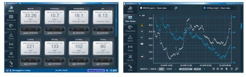
It receives UV/VIS absorption spectrums and via integrated algorithms, it detects events.
